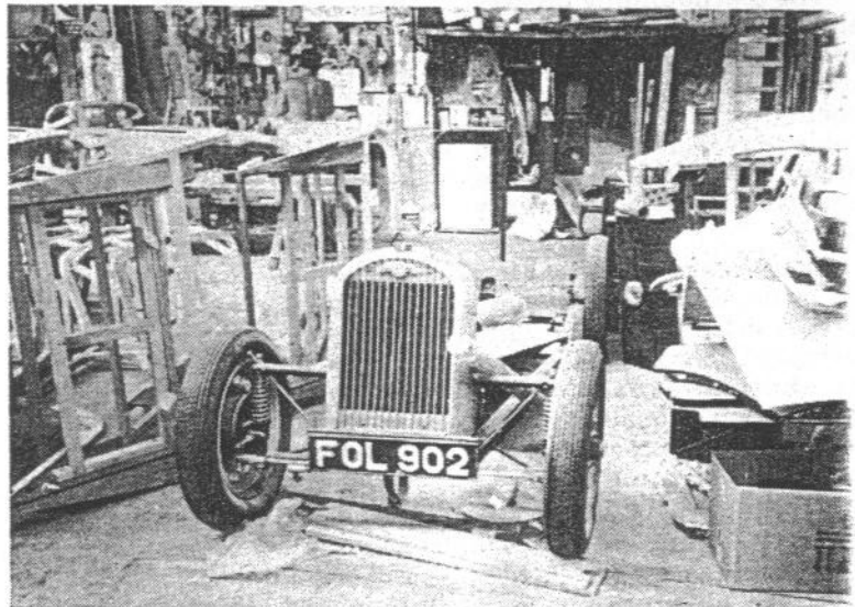
The simple, ingenious sliding-pillar front suspension has barely changed since 1909. The setup on a brand new 1995 chassis closely resembles that on a late-1930s model.
